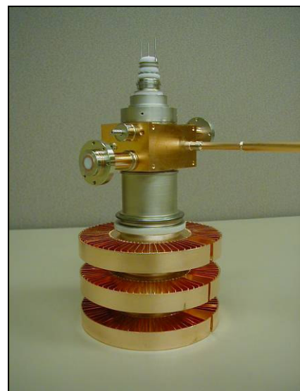
Figure 4. The MSDC Ka-Band EIK vacuum assembly
