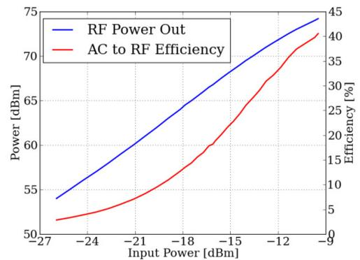
Figure 4: Output power and efficiency vs. input RF power.
