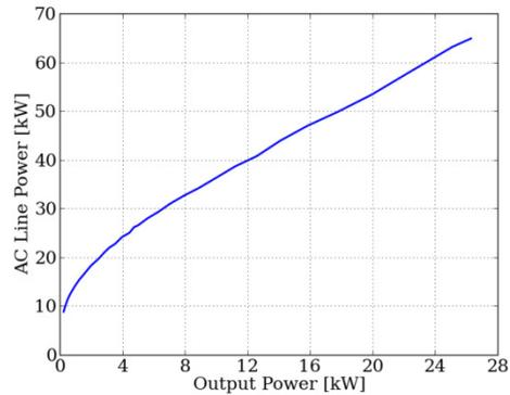
Figure 9: AC line power vs. output power.
