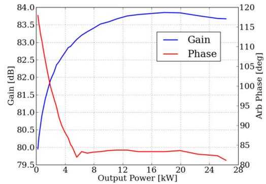
Figure 3: Gain and phase vs. output power.
