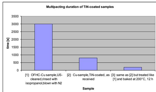
Figure 2: Results of DESY measurements on CPI samples showing multipacting duration of TiN-coated samples. Data provided by Arne Brinkmann of DESY.
