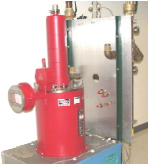
Figure 5: VKL-7966A Klystron in Electromagnet (Photo courtesy of TJNAF)
