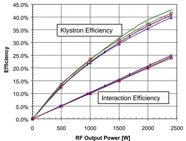
Fig. 5. Measured interaction and klystron efficiency vs. rf output power for serial numbers 100 ( $\diamond$ ), 102 ( $\square$ ) and 103 ( $\triangle$ ). The theoretically expected klystron efficiency ( $\%4$ ) is shown as well.
