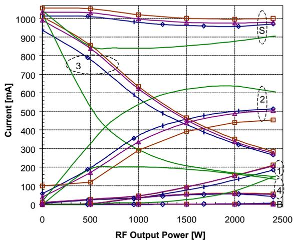
Fig. 3. Power supply current (S), collector current splits (1, 2, 3, 4) and body current (B) of the VKU-8891 vs. rf output power. The diagram shows measured data of serial numbers 100 ( $\diamond$ ), 102 ( $\square$ ), 103 ( $\triangle$ ) and theoretical values ( $\%4$ ).
