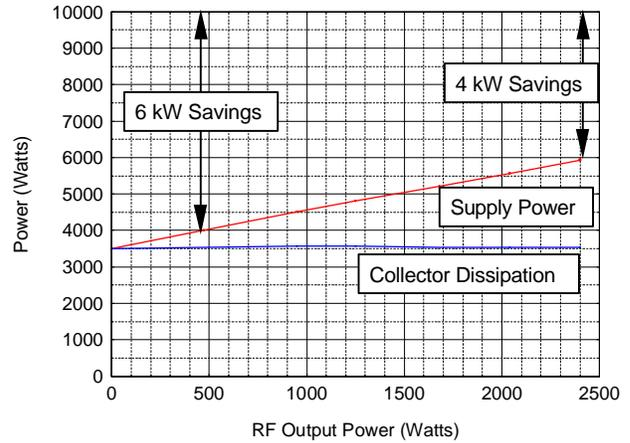
Fig. 4. Required supply power and dissipated power vs. rf output power measured for serial number 100 at a frequency of 17.5 GHz. The arrows indicate the energy savings in comparison to a grounded collector.
