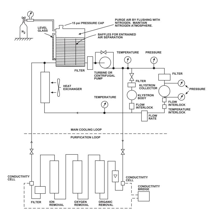
Figure 1. KLYSTRON COOLING SYSTEM WITH PURIFICATION LOOP
