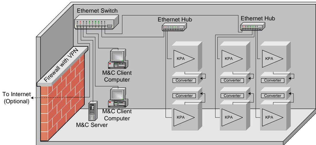
Figure 1 - Example of Ethernet Earth Station Wiring
