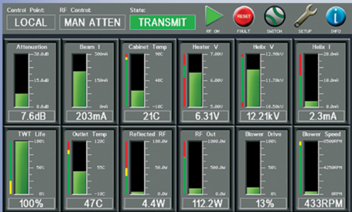
Figure 4. LIFEEXTENDER/LIFEPREDICTOR GUI screen. The remaining TWT life is shown in the lower left hand box.
