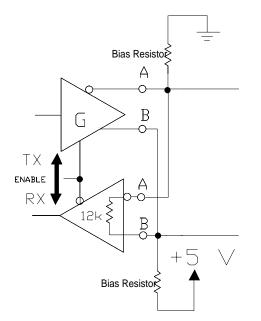
Figure 2.4 Transceiver with Bias Resistors
