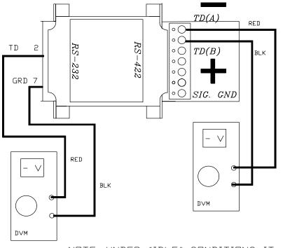
NDTE: UNDER "IDLE" CONDITIONS IT IS POSSIBLE TO DETERMINE WHICH TERMINAL IS "A" AND WHICH IS "B"
