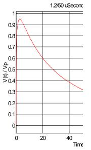
Figure 4.1 Combination Wave Voltage Waveform
