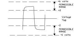
BALANCED DIFFERENTIAL DUTPUT LINE DRIVER
