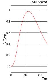
Figure 4.2 Combination Wave Current Waveform
