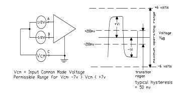
BALANCED DIFFERENTIAL INPUT LINE RECEIVER
