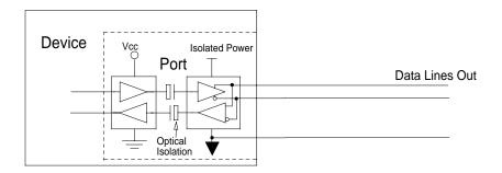
Figure 4.4 Isolated RS-485 Device
