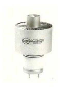
The 3CX2500D3 is a forced air cooled, ceramic/metal, medium-mu power triode designed primarily for use in industrial radio frequency heating services. Input of 7.77 kW is permissible up to 110 MHz. Plentiful reserve emission is available from it's 233 watt filament. The grid structure is rated at 75 watts making this tube an excellent choice for industrial service.
