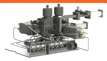
Typical Ku-Band 1:2 LNB Plate Assembly
