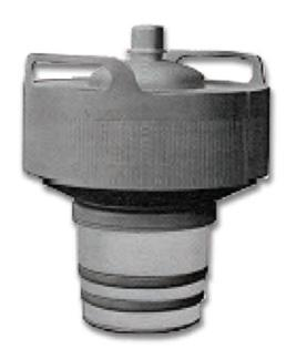
The 4CX15,000A/8281 is intended for use in audio or radio frequency applications. It features a new type of internal mechanical structure which results in high RF operating efficiency. Low RF losses in this mechanical structure permit operation of the 4CX - 15,000A/8281 at full ratings up to 110 MHz and at reduced ratings to 225 MHz.
