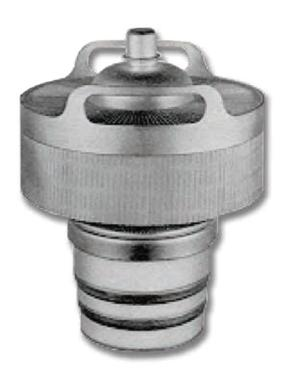
The 4CX10,000D/8171 is identical to the 4CX5000A/8170 except for its rated plate dissipation. Its increased capability, resulting in a larger cooler, is most useful in linear applications where plate dissipation is generally the limiting factor. The larger cooler also allows the 4CX10,000D/8171 to be used in place of the 4CX5000A/8170 with cooler operation at any given air flow rate.
