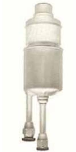
The 3CW5000A7 is a water-cooled high-mu triode intended for use as an RF amplifier in industrial applications where water cooling is preferred over air cooling. This tube is a water-cooled version of the 3CX3000A7.
