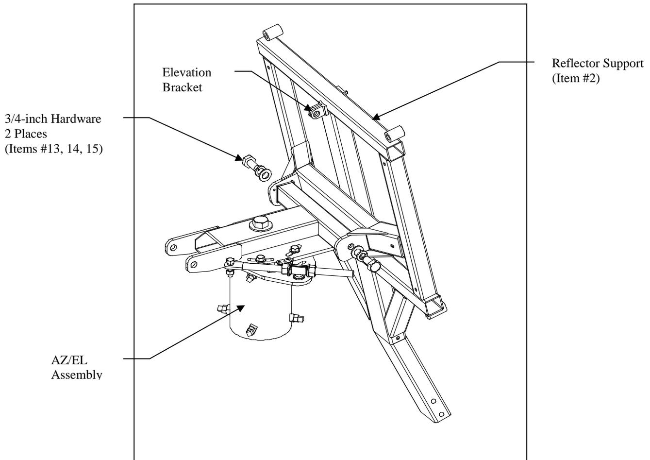
3. Attach the elevation adjustment rod (Item #4) to the elevation mounting bracket of the reflector support with the elevation pivot sleeve,  $\frac{1}{2}$ -13 x 1.75-inch bolt, two flat washers, and hex nut (Items #6, 8, 9, 10, 11).
