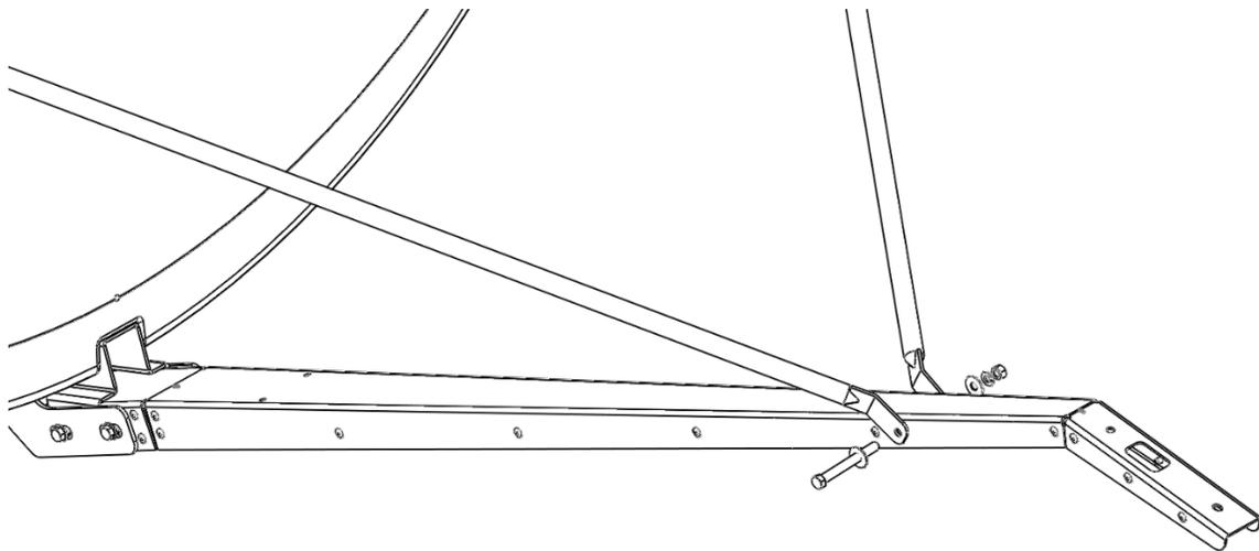
7. Tighten securely the three 5/16-inch bolts used to attach the feed system to the reflector and the 5/16-inch bolt used to attach the feed rods to the feed support at this time.
