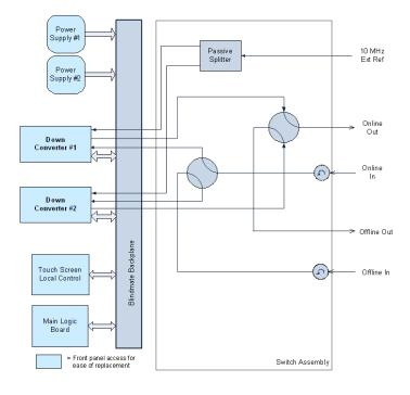
1 for 2 (1:2) Redundant Downconverter System
