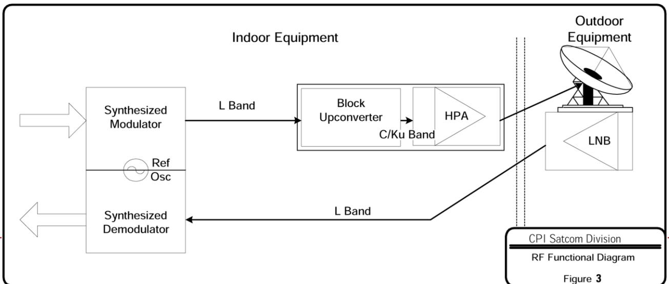
integrated into an indoor rack mount HPA, it can also be integrated into CPI's hub mount HPA products.
