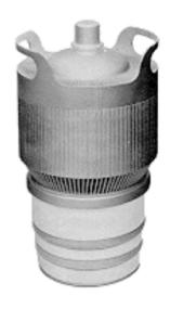
The 4CX5000A/8170 is useful as an oscillator, amplifier or modulator at frequencies up to 220 MHz, Class AB<sub>1</sub> audio amplifier, or as a screen-modulated radio frequency amplifier. The rated plate dissipation is 5 kW for most classes of service and 6 kW for Class AB operation.
