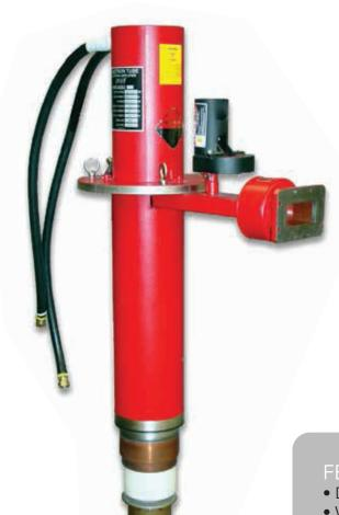
CPI Microwave Power Products (MPP) offers the VKS-8262 series of klystrons for use in particle accelerators for scientific, medical, and industrial applications. These klystrons provide up to 7.5 MW peak at 2.856 or 2.9985 GHz at various rf pulse lengths and duty. Versions are available with up to 36 kW of average output power at 2.856 GHz and 72 kW at 2.9985 GHz.
