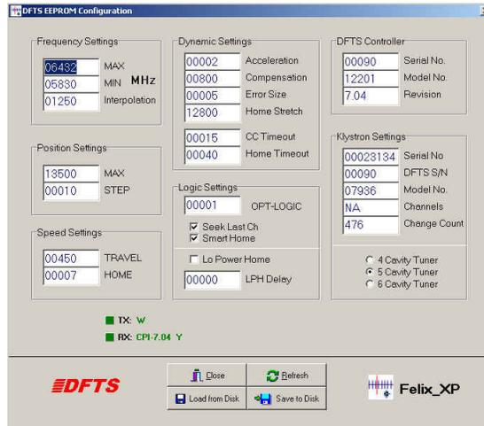
Accessed by clicking the [Access Menu] button from the Channel Database dialog, and selecting [EEPROM Configuration] or from the main menu by selection [Tuning]-[EEPROM Configuration].
