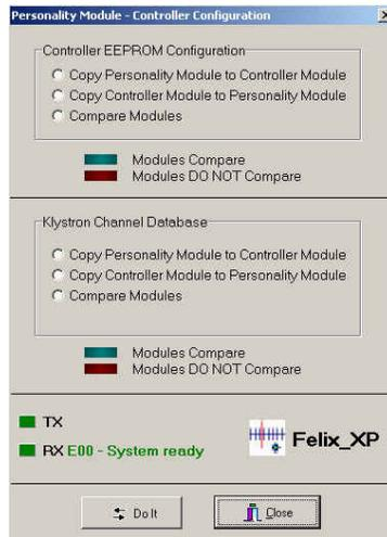
This permits you to compare the DFTS Controller Module (CM) software parameters and klystron database parameters to those in the Klystron Personality Module (KPM). It also permits you to copy the data from either the CM to the KPM, or KPM to the CM
