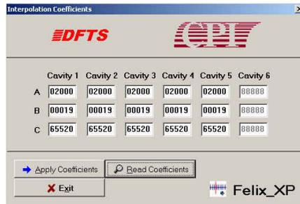
This dialog displays the Interpolation Coefficients used in Parabolic Frequency Interpolation. It allows you to read and write the coefficients to the DFTS.
