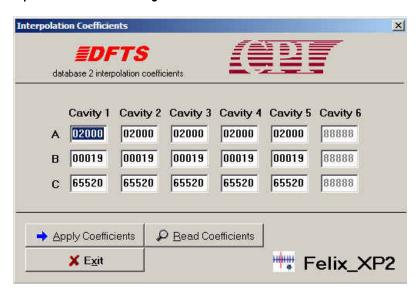
This dialog displays the Interpolation Coefficients used in Parabolic Frequency Interpolation. It allows you to read and write the coefficients to the DFTS.
