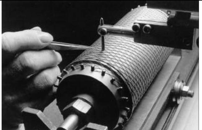
The original tube design establishes the overall performance characteristics. Replacement parts exactly duplicate the original parts in form, fit, and function. Jigs and fixtures aid in the production and assembly, but skilled tube technicians are the brains and hands that do the job.
