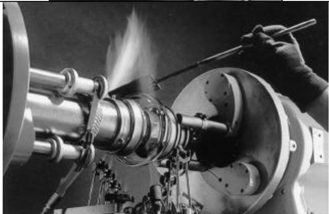
Tubes with cracked ceramics were previously considered unrebuildable. Here, a 4CX3500A is prepared to have the cracked output ceramic removed and replaced.
