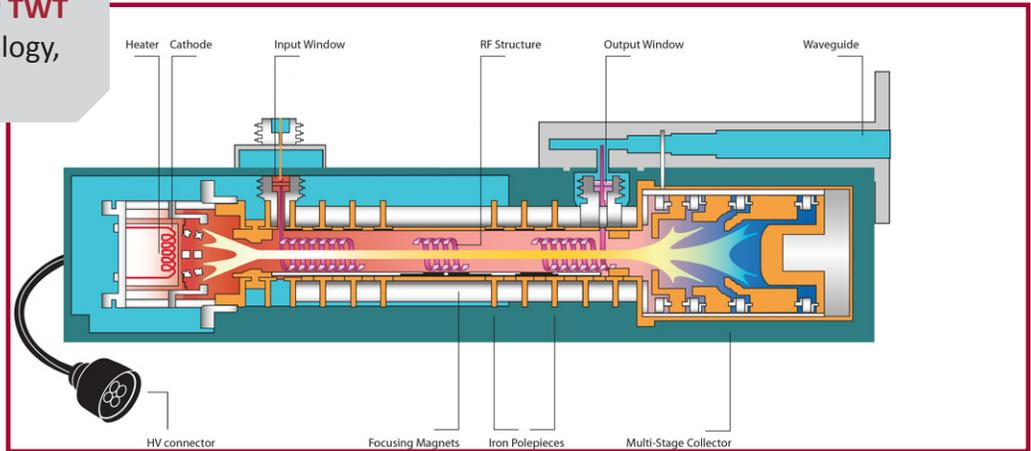
CPI's *LIFEEXTENDER* is new, patented technology which is a leap forward over other methods introduced to the satcom amplifier market to increase traveling wave tube (TWT) life. CPI's dynamic *LIFEEXTENDER* is the only method where the life of the TWT is extended by preserving the active coating on the cathode surface.
