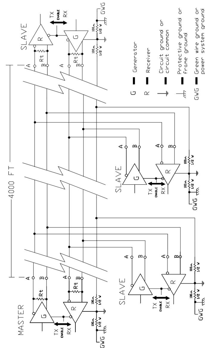
Figure 2.1 Typical RS-485 Four Wire Multidrop Configuration
