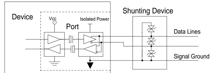
**Figure 4.8 Isolated port with ungrounded shunt protection**
