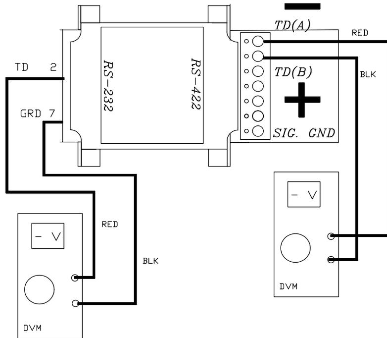
NOTE: UNDER "IDLE" CONDITIONS IT IS POSSIBLE TO DETERMINE WHICH TERMINAL IS "A" AND WHICH IS "B"
