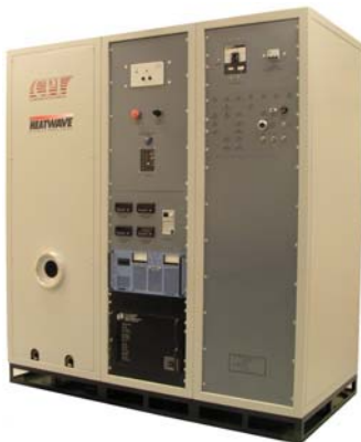
10 KW, 28 GHz, Laboratory enclosure
