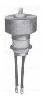
The 3CX15,000H3 is a forced air cooled, ceramic/metal, medium-mu power triode designed primarily for use in industrial radio frequency heating services. Input of 56.2 kW is permissible up to 90 MHz. Plentiful reserve emission is available from it's 1000 watt filament. The grid structure is rated at 500 watts making this tube an excellent choice for industrial service.
