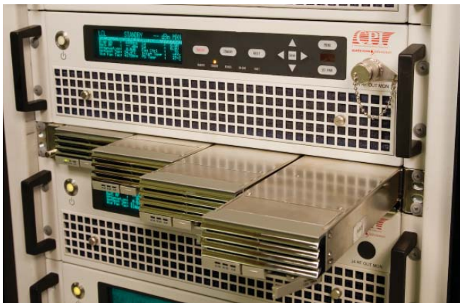
SSPA with redundant hot-swappable power supplies (optional with 100 W SSPA, required with 200 W SSPA)
