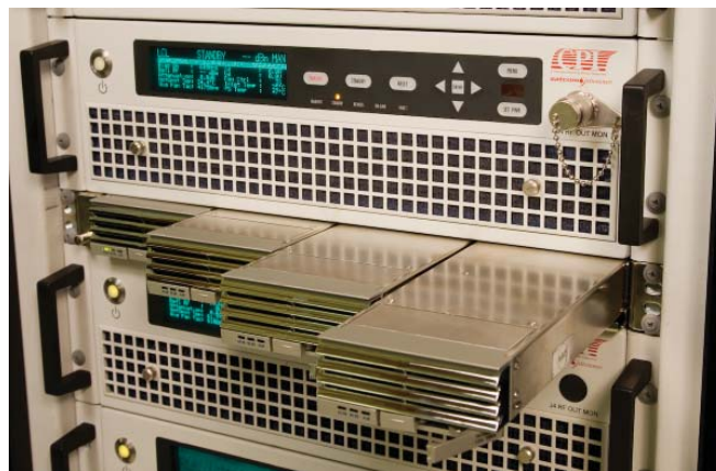
SSPA with optional redundant hot-swappable power supplies
