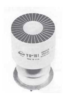
The 3CX1200Z7/YU-181 is a high mu, forced air cooled rugged ceramic triode intended for use as a grounded grid, zero bias Class AB<sub>2</sub> amplifier.
