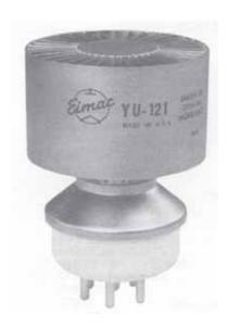
The 3CX1200D7/YU-121 is a high mu, forced air cooled rugged ceramic/metal power triode intended for use as a grounded grid, zero bias Class AB<sub>2</sub> amplifier.
