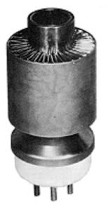
The 3CX1200A7 is a high mu, forced air cooled rugged power triode intended for use as a zero bias Class  $AB_2$  RF amplifier to 110 MHz.
