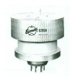
The 8295A is a radial beam pentode intended for use as a linear amplifier. The anode is forced-air cooled and has a maximum dissipation rating of one kilowatt.
