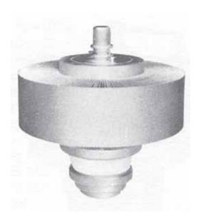
The 3CX10,000U7 high-mu triode is intended for use as a cathode driven RF amplifier in the VHF specturm. It is a very linear device making it ideally suited for TV service in addition to CW and pulsed RF amplifer service. The 3CX10,000U7 makes use of beam forming cathode and control grid geometry to product high gain, low grid interception and zero-bias operation capability. The CV2240B and CV2250B 10 kW peak sync VHF-TV broadcast cavities are available for use with the 3CX10,000U7.
