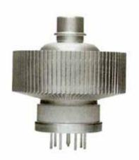
The YC-236 is a selected 8877/3CX1500A7 certified for use as a cathode-driven Class B amplifier in FM transmitter applications. Sample testing is performed periodically in a 2 kW FM transmitter at the Eimac factory.
