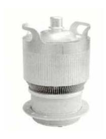
The 3CX5000A7 high-mu triode is designed for use as a cathode driven Class AB power amplifier. The tube does not require a socket as it is designed to bolt directly to the chassis by means of the grid flange. Cathode and heater connections are made by bolting directly to the amplifier circuitry. These features reduce equipment cost and complexity.
