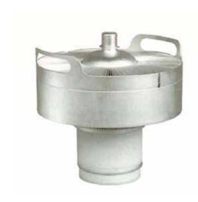
The 3CX20,000A7 is a high-mu power triode intended for use as a zero bias Class B RF amplifier or Class C power amplifier or oscillator. Class B operation with zero grid bias offers circuit simplicity. In addition, grounded grid operation is attractive since a power gain as high as twenty times can be obtained.
