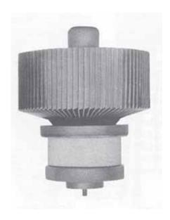
The 3CX1500C7/8938 is a rugged coaxial base power triode designed for use as a cathode-driven Class AB<sub>2</sub> or Class C amplifier. It is recommended for VHF or UHF service as a linear amplifier, power amplifier or pulse amplifer. Linearity and power gain are both excellent due to the low ratio of gridto-plate current and relatively high amplification factor. Low grid interception of available emission current is due to the beam forming geometry of the special grid and cathode design.
