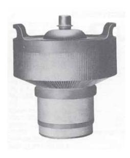
The 3CX10,000A7/8160 is a high-mu power triode intended for use as a zero bias Class B amplifier an audio or RF applications, or as a Class C amplifier, CW or modulated. Operation in a Class B with zero grid bias offers circuit simplicity by eliminating the bias supply, and in addition, grounded grid operation is attractive since a power gain as high as twenty times can be obtained with the tube.
