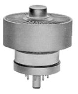
The 8930 is electrically identical to the 4CX250R/7580W, but the larger anode radiator assembly allows higher dissipation with low air flow and pressure drop characteristics. The tube has rugged internal construction features for reliable operation under heavy shock and vibration conditions.
