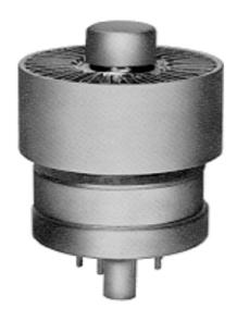
The 4CX350F/8322 has a maximum plate dissipation of 350 watts and is intented for Class AB audio or RF amplifier service. The tube is externally identical to the 4CX250B but contains rugged internal construction features. Amplification factor and cathode area have been increased over the basic 4CX250B to give higher transconductance and figure of merit.
