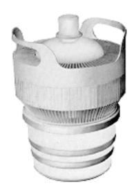
The 4CX3500A is a compact power tetrode designed to be used in VHF power amplifier service. It features a type of internal structure that results in high RF operating efficiency up to 220 MHz. This tube is also recommended for use as a VHF TV linear amplifier, for use as a Class C radio frequency power amplifier and plate-modulated radio frequency audio amplifier.
