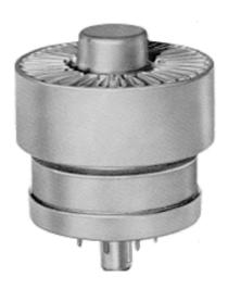
The 4CX250B/7203 has a maximum plate dissipation rating of 250 watts and a maximum input power rating of 500 watts. The 4CX250B/7203 is designed to operate with a heater voltage of 6.0 volts.
