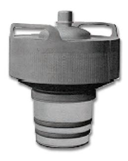
The 4CX15,000R is identical to the 4CX-15,000A except that it has a mesh filament. The mesh filament is particularly well suited to FM service at 108 MHz due to reduced filament inductance. It is also recommended for VHF TV linear amplifier service to 225 MHz.
