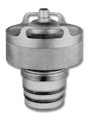
The 4CX10,000J has a rated maximum plate dissipation of 12 kW. It incorporates rugged internal construction features including a mesh filament. The 4CX10,000J is specifically designed for low intermodulation distortion in radio frequency linear amplifier service.
