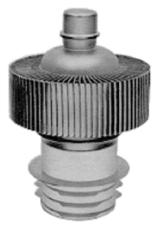
The 4CX1500B/8660 is a low voltage, high current tetrode specifically designed for exceptionally low intermodulation distortion and low grid interception. The low distortion characteristics make the 4CX1500B/8660 especially suitable for radio frequency and audio frequency linear amplifier service.
