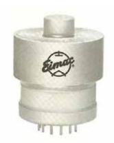
The 3CX400A7/8874 is a compact high-mu power triode intended for use in zero bias Class B amplifiers in audio or RF applications. Operation with zero bias simplifies circuitry and cathode driven operation is attractive since a power gains as high as twenty can be obtained.
